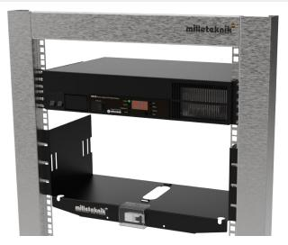
The battery shelf must be mounted in a 19" rack. Use the appropriate screw for the rack to attach the shelf.
