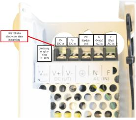
Connect voltage and load on the power supply.
